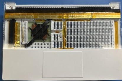
Fig. 7: Thermal Test Vehicle (TTV) consisting of the laptop base with the integrated thermal module.
