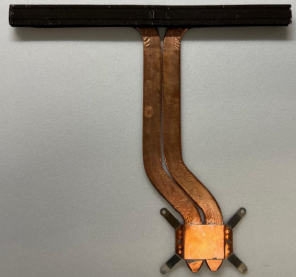
Figure 2: Thermal module with the fins stack coated with \text{MnO}_2 (Shown in black).
